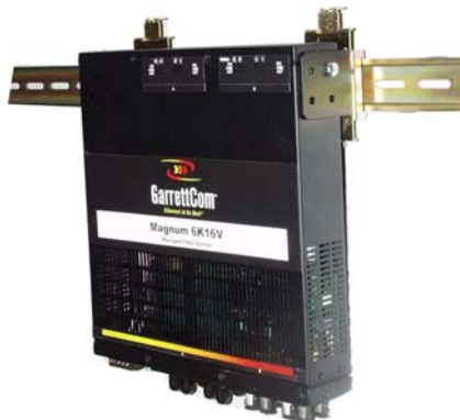
Magnum 6K16V mounted vertically with DIN-Rail brackets and latches
